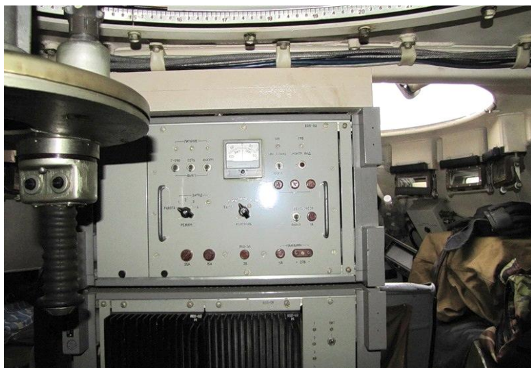
Fig. 5. Operating panel of ZS-82 (“The Decorator”).
