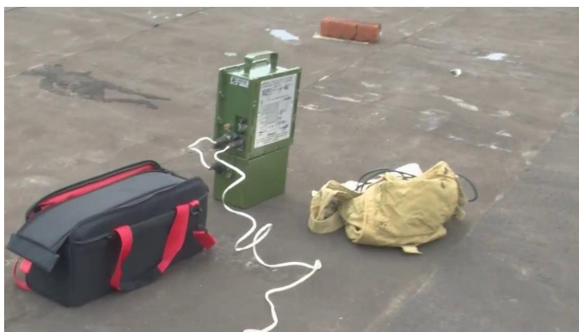
Fig. 1. Lightweight sound broadcasting station – OZS-78
