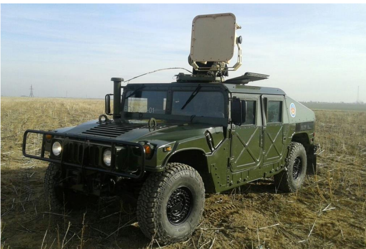
Fig. 3. Vehicle sound broadcasting station based on “Hummer” off-road vehicle.
