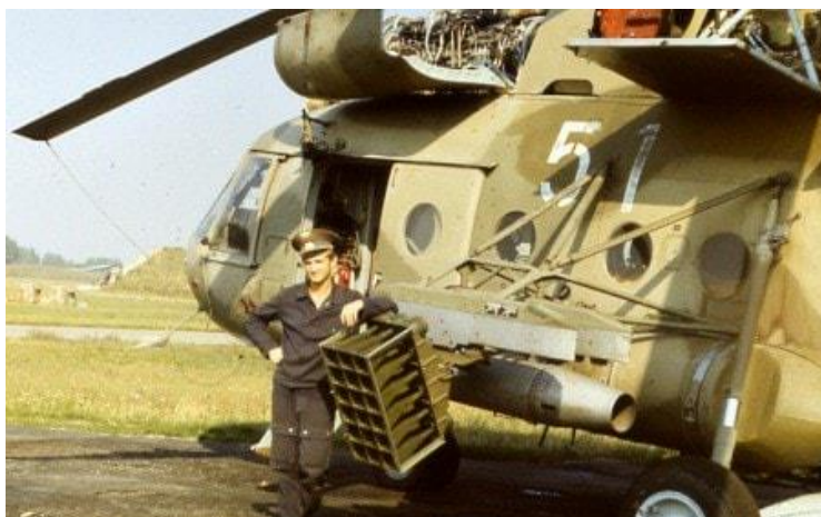
Fig. 6. Soviet sound broadcasting station placing in a helicopter
